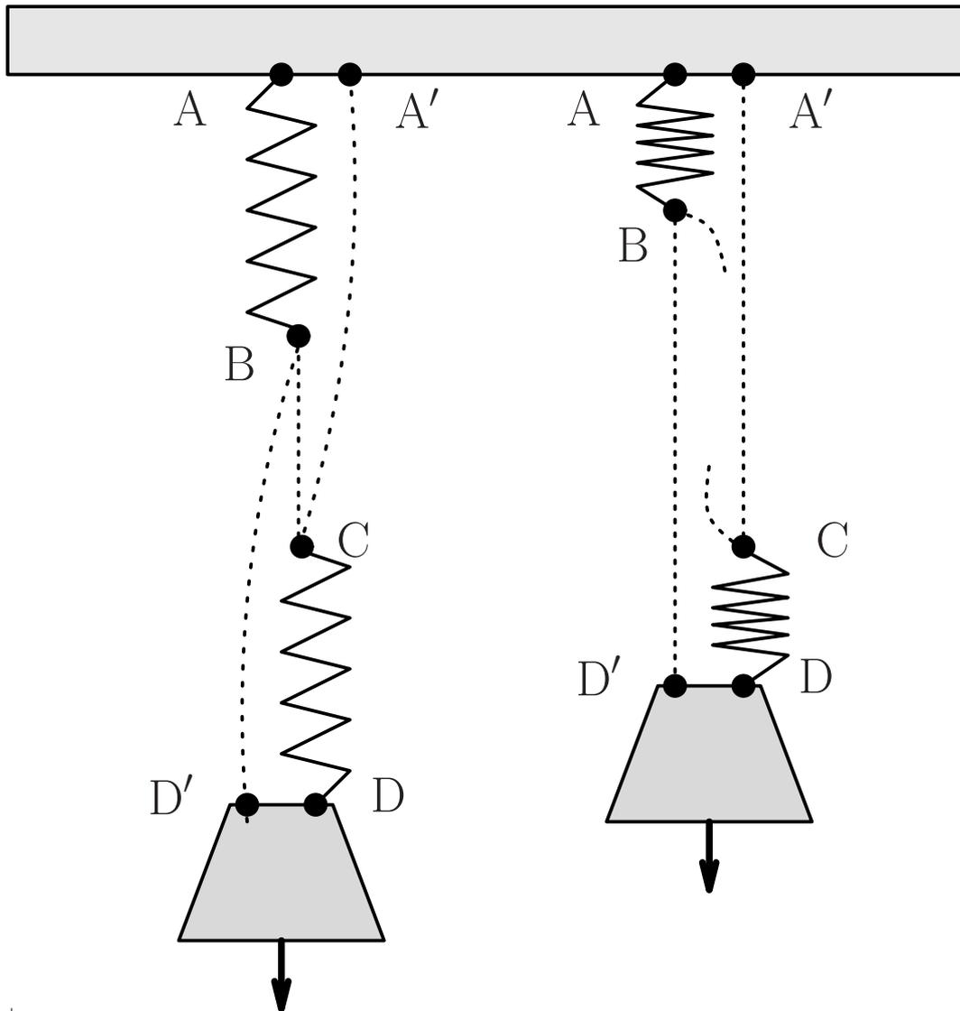
Springs of equal strength are stretched AB and CD. Strings A'C and BD' (shown as dotted) are initially 'just slack'.
