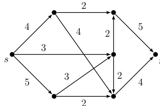
**12.** Explain how the Ford–Fulkerson algorithm can be used to find a maximum flow in an undirected network. Find a maximum flow from  $s$  to  $t$  in the following network, and prove that it is indeed optimal:
