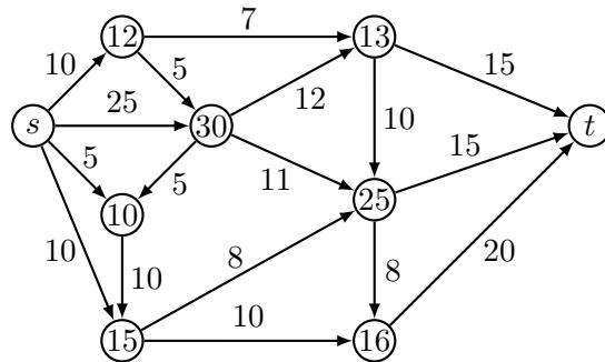
Determine the maximum flow from  $s$  to  $t$ . Suppose that the capacity constraint of one of the intersections could be removed completely by building a flyover. For which intersection should this be done in order to increase the maximum flow as much as possible?
