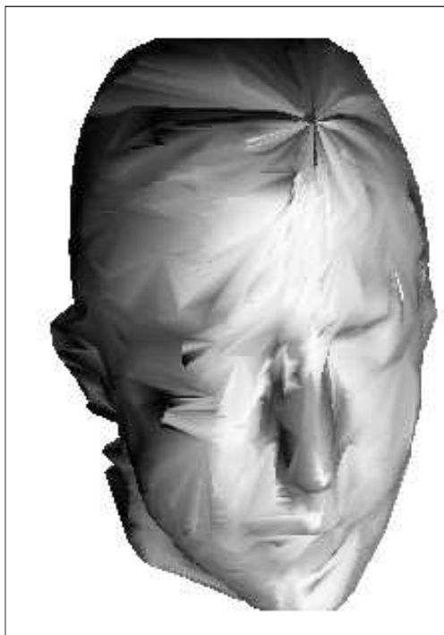
Figure 4.9: Vicki approximated by the sophisticated thickness calculation. \epsilon = 2\text{cm} , 2979 vertices and 5861 triangles.
