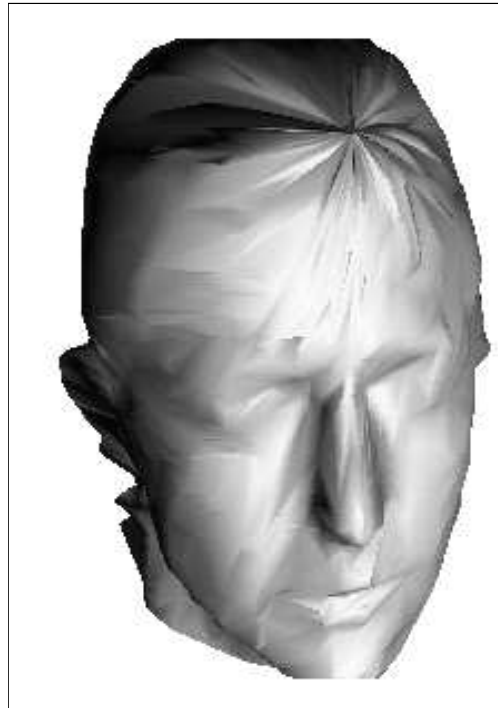
Figure 4.11: Sophisticated, random approximation. \epsilon = 0.5 , 1741 vertices and 3391 triangles
