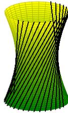
FIGURE 1. Lines on the hyperboloid of one sheet
